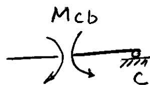
$$\boxed{\begin{aligned} M_{ba} + M_{bc} &= 0 \\ M_{cb} &= 0 \end{aligned}} \quad \text{--- } ②$$
